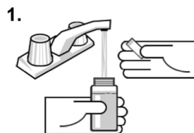
Figure 1 - From Tap: Hold cap in one hand while filling the sample bottle with the other.
